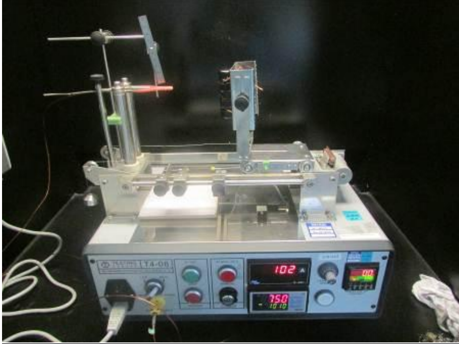
Photo 1: Positioned tested sample on testing apparatus (750°C) – I connector
