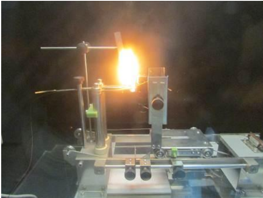
Photo 2: There is flame (during test at 750°C) – I connector
