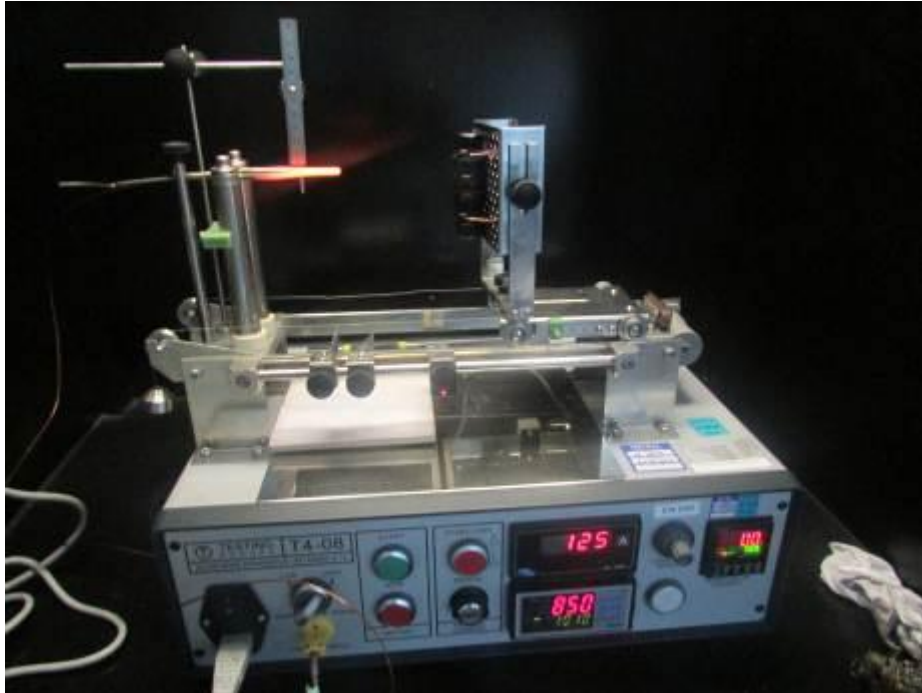
Photo 4: Positioned tested sample on testing apparatus (850°C) – I connector
