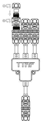
3) Tightening torgue 0,5Nm Cross-Slotted head screwdriver DIN ISO 8764
